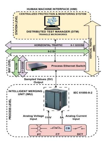
PT: Potential Transformer CT: Current Transformer CB: Circuit breaker DCT: Disconnector
